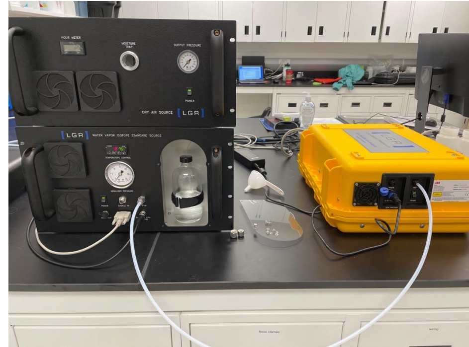
Los Gatos Research (LGR) Portable Water Vapour Isotope Analyzer (field deployable)
